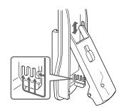
· Install the hook to face side ways if the fin of the air conditioner is vertical.
