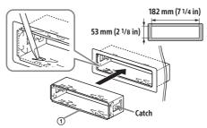
**2** Mount the unit onto the bracket ①, then attach the protection collar ③.
