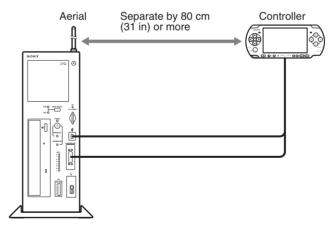
When using the wireless LAN function, separate the unit's aerial and the controller by at least 80 centimeters (31 inches). Alternatively, you can use the Network Kit (DTP-H120) (sold separately). If the unit is used with the controller and aerial in close proximity to each other, radio frequency interference from the controller will interfere with the wireless LAN signal and can cause an increase in loss of data packets.
