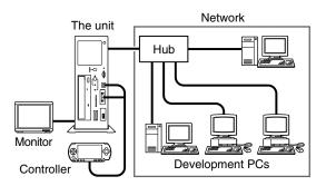
In this case, the IP address and subnet mask settings will be obtained automatically when the unit is turned on. Depending on the settings of the DHCP server, other network settings, such as the DNS server and default gateway, may also be obtained. For details on which settings can be automatically obtained, contact your network administrator.
