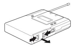
2 Insert new batteries, making sure the polarities are correct, and then return the battery holder to its original position.
