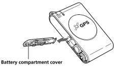
If the battery compartment cover comes off, align the hinge tabs of the battery compartment cover to the hinge clasps of the unit, and gently snap the cover into place.
