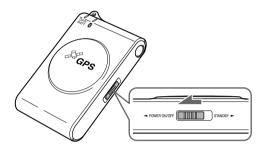
The power switch returns to the STANDBY position automatically when you release it.
