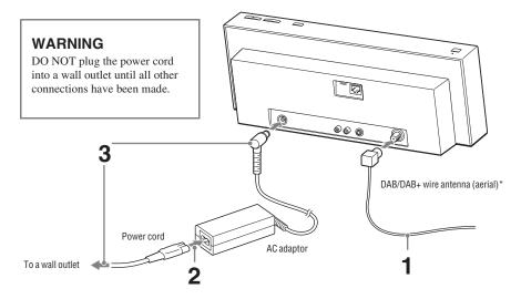
\* The DAB/DAB+ wire antenna (aerial) and the ANTENNA DAB 75  $\Omega$  are available for the UK model only.
