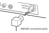
Use an external DAB/DAB+ antenna for a more robust DAB/DAB+ signal. It is recommended you only use the supplied DAB/DAB+ wire antenna for areas of strong DAB/DAB+ reception or as a temporary measure until you install an optional external antenna.
