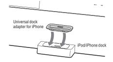
To remove the universal dock adapter for iPhone, pull it up with your fingernail or a flat object using the slot inside the adapter.
