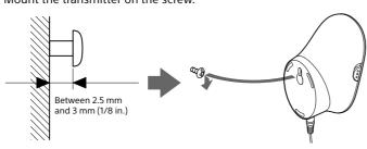
The transmitter clicks when it is turned to the maximum angle. Do not try to turn it any further • When mounting the transmitter on a wall, use the screw suitable to the wall material or strength. Attaching screw may damage the wall. Attach the screw firmly to a pillar or a stud in a wall, if possible.
