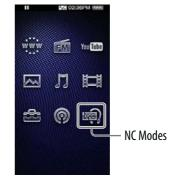
Connect the supplied headphone to the player and slide the NOISE CANCELING switch in the direction of the arrow ►.
