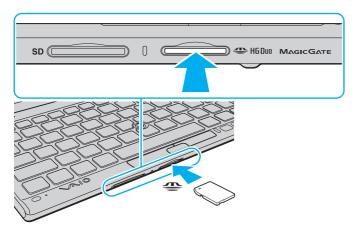
Before using "Memory Stick Micro" ("M2"), be sure to insert it into an "M2" Duo adaptor. If you insert the media directly into the "Memory Stick Duo" slot without the adaptor, you may not be able to remove it from the slot.
