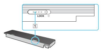
**3** Fit the battery pack into the battery compartment. The battery pack should be level with the bottom of the computer.
