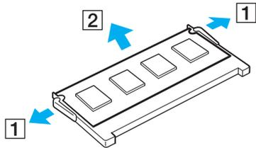
□ Make sure that the memory module tilts up and then pull it out in the direction of the arrow (2).
