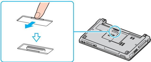
5 Align the bottom connector of the computer with the connector on the port replicator and push down until it clicks into place.
