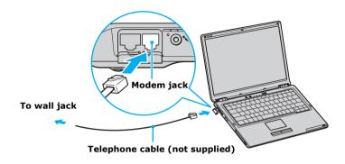
Your computer does not work with party lines, cannot be connected to a coin-operated telephone, and may not work with multiple telephone lines or a private branch exchange (PBX). Some of these connections may result in excess electrical current and could cause a malfunction in the internal modem.
