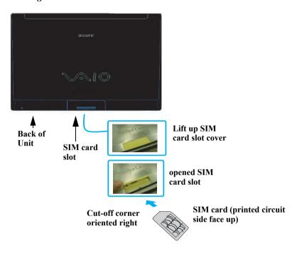
If your computer came with a preinstalled Cingular SIM card, verify that the card is indeed in the SIM card slot.
