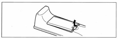
2. Install two AA type batteries. See below polarity of each battery.
