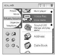
**2** Press the VOICE REC button. The recording starts. Speak into the built-in microphone.
