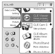
3 Rotate the Jog Dial<sup>™</sup> navigator to select the file you want to display and press the Jog Dial<sup>™</sup> navigator.
