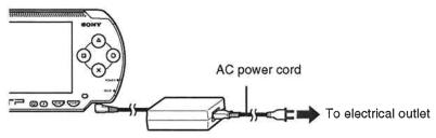
The power indicator lights up in orange, indicating that charging has begun. The power indicator will turn off when the battery is fully charged.
