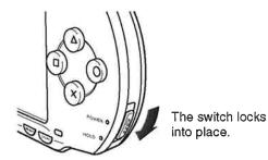
The hold indicator turns yellow, indicating that the system buttons are locked.
