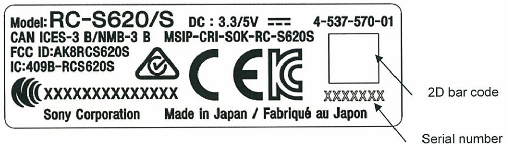
Figure 2-4: Contents of spec indication label
