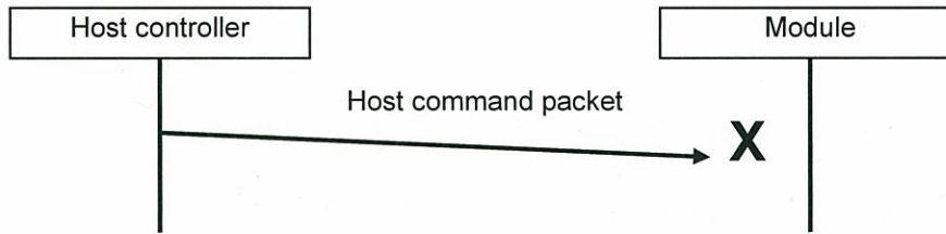
Figure 3-2: Data link level error in host command packet
