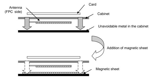
Figure B-2: Reduction of the impact of metal
