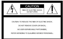
This symbol is intended to alert the user to the presence of uninsulated "dangerous voltage" within the product's enclosure that may be of sufficient magnitude to constitute a risk of electric shock to persons.
