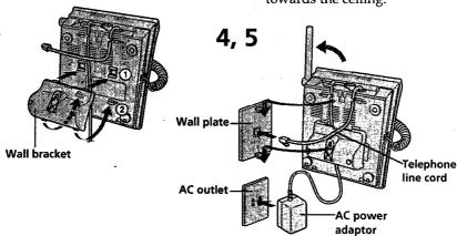
**Tip**To remove the wall bracket, press the lower tabs.
