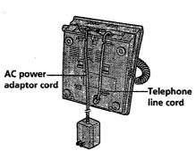
Attach the wall bracket to the center of the base phone.
