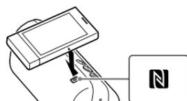
Complete the connection by following the instructions on the screen. When the BLUETOOTH indicator (blue) stops flashing and remains lit, the unit is connected with the device. To disconnect the unit, touch it with the smartphone again.
