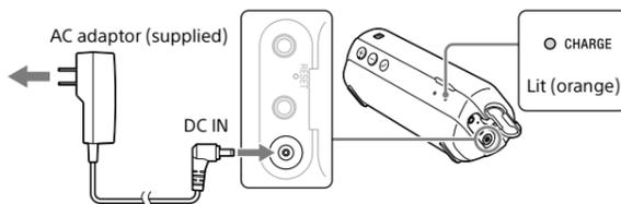
Charging starts when the unit is connected to an AC outlet via the AC adaptor, and the CHARGE indicator (orange) lights up. Charging is completed in about 3 hours and the indicator goes off.
