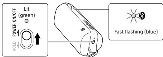
**2 Perform the pairing procedure on the BLUETOOTH device to detect this unit.**
