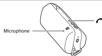
Operate your mobile phone to make a call. To terminate a call, press the button on the unit.
