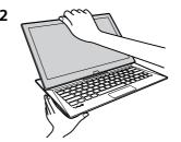
Grasp the top center edge of the LCD screen and raise it to use the keyboard.
