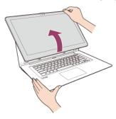
4. Move the LCD screen in the direction of the arrow to fold the screen. The LCD screen is folded on the keyboard.
