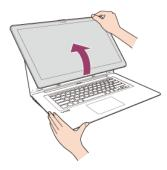
Move the LCD screen in the direction of the arrow to fold the screen. The LCD screen is folded on the keyboard.
