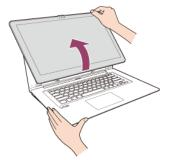
4. Move the LCD screen in the direction of the arrow to fold the screen. The LCD screen is folded on the keyboard.
