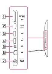
1 "Memory Stick Duo" / SD memory card combined slot "Memory Stick Duo" and an SD memory card cannot be inserted into the slot simultaneously.
