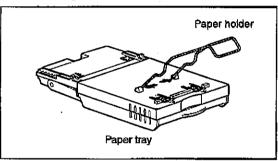
Push the paper holder into the stoppers firmly until it snaps into place, making a click sound.
