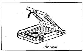
Riffle the print paper. Then insert the print paper with its printing surface (the side with no imprint) facing up and the arrow pointing in the same direction as the arrow in the tray.
