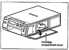
2 Insert the print cartridge into the printer firmly until it clicks into place.
