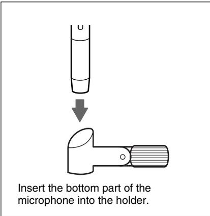
Insert the bottom part of the microphone into the holder.
