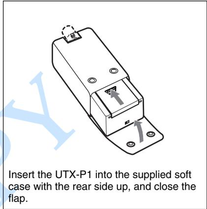
Insert the UTX-P1 into the supplied soft case with the rear side up, and close the flap.
