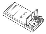
**3** Be sure to line up the + and - of the batteries and insert the two supplied size AA (LR6) alkaline batteries.
