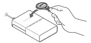
The LOCK and UNLOCK indicators flash alternately, then the wireless key is registered to the drive.
