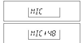
**3** Press the + button to select the setting "MIC+48", or press the – button to select the setting "MIC"
