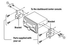
When mounting this unit to the preinstalled brackets of your car, use the supplied screws () in the appropriate screw holes based on your car: T for TOYOTA and N for NISSAN.
