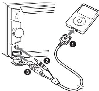
While the iPod is connected, a device connected to the front AUX terminal becomes unavailable, and “Front AUX” cannot be selected when changing the source.
