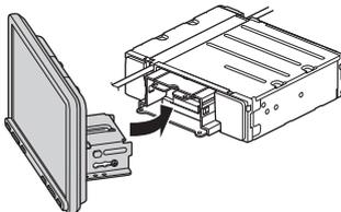
Make sure that the connector brackets of the display is fully inserted to the unit.
