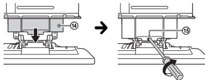
When you tighten a screw, be careful not to apply too much torque as doing so may damage the screw (the torque value should be less than 1 N•m).
