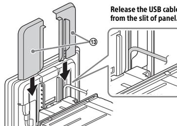
Release the USB cable from the slit of panel.
