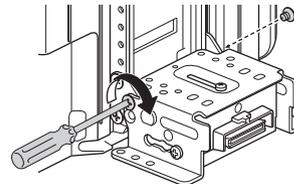
When you tighten a screw, be careful not to apply too much torque as doing so may damage the screw (the torque value should be less than 1 N•m).
