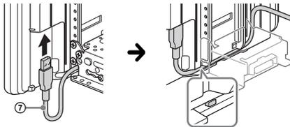
To prevent the extension cable from coming off, be sure to route the USB cable along the groove through the catches inside.
