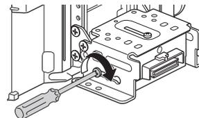
When you tighten a screw, be careful not to apply too much torque as doing so may damage the screw (the torque value should be less than 1 N•m).
