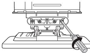
When you tighten a screw, be careful not to apply too much torque as doing so may damage the screw (the torque value should be less than 1 N•m).
