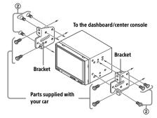
When mounting this unit to the preinstalled brackets of your car, use the supplied screws (2) in the appropriate screw holes based on your car: T for TOYOTA, M for MITSUBISHI and N for NISSAN.
