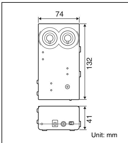
$132 \times 41 \times 74 \text{ mm } (5 \frac{1}{4} \times 1 \frac{5}{8} \times 3 \text{ inches})$  (w/h/d)
