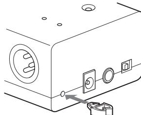
Insert the cable clamp into the cable clamp attachment hole on the left side of the receiver.
