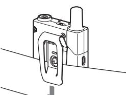
Slide the guitar strap into the belt clip on the unit completely, and make sure it is secure.
