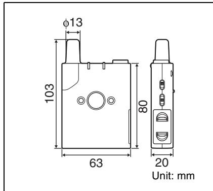
$63 \times 80 \times 20 \text{ mm } (2 \frac{1}{2} \times 3 \frac{1}{4} \times \frac{13}{16} \text{ inches})$  (w/h/d) (excluding the antenna)
