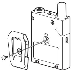
Align the mounting hole at the rear of the transmitter with the hole in the middle of the supplied belt clip, and secure the belt clip using the supplied belt clip screw. You can also rotate the belt clip 180 degrees or 90 degrees to the left or right before securing it.
