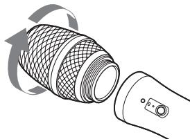
Turn the microphone unit in the direction of the arrow.
