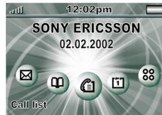
There are five application shortcuts in the standby view. The selected application is highlighted and its name is shown at the bottom left of the screen above the OK key. Press **Jog Dial** or OK to start the application.
