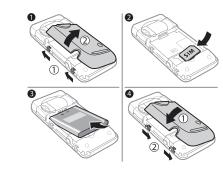
Slide the catches to the left and lift the battery cover side as shown in the picture. Remove the battery cover by tilting it until the hinges on the battery cover side release.
