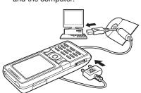
2 Phone: Select File transfer or ▶ Settings ▶ the Connectivity tab ▶ USB ▶ USB connection ▶ File transfer. The phone shuts down.
