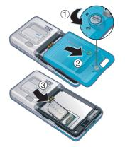
1 Unlock the battery cover by screwing the cover lock as shown in the picture.
