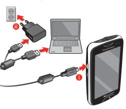
Connect the phone to a power outlet using the USB cable and the power adapter.
