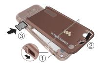
Open the cover and insert the memory card with the gold-coloured contacts facing down.
