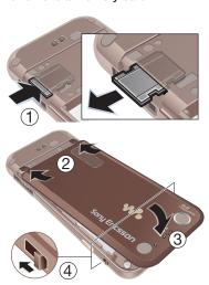
Open the cover and press the edge of the memory card to release and remove it.
