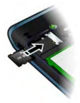
Open the cover and insert the memory card with the gold-coloured contacts facing down.
