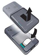
Remove the battery cover by pressing and sliding it as shown in the picture.
