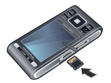
Open the cover and insert the memory card with the gold-coloured contacts facing up.
