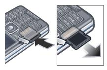
· Open the cover and press the edge of the memory card to release and remove it.
