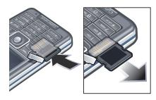
Open the cover and press the edge of the memory card to release and remove it.
