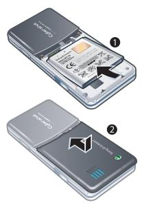
1 Insert the battery with the label side up and the connectors facing each other.
