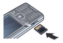
Open the cover and insert the memory card with the gold-coloured contacts facing up.
