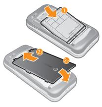
1 Insert the battery with the label side up and the connectors facing each other.
