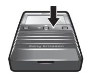
Press the navigation key upwards, downwards, left or right to move through the menus
