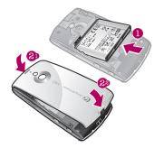
1 Insert the battery with the label side up and the connectors facing each other.
