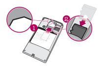
• Slide in the SIM card and the memory card with the goldcoloured contacts facing down.
